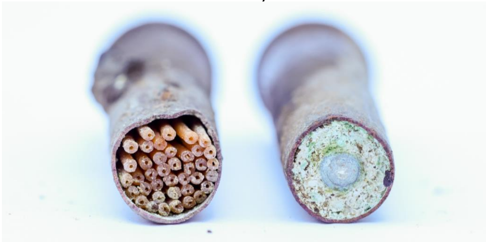
Figure 5-18: Internal view of the cordite and wadding internal to the firing mechanism within the ammunition cartridges.
